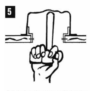
Push the firehood as far as possible into the hole using a blunt object so it is fully open in all directions
